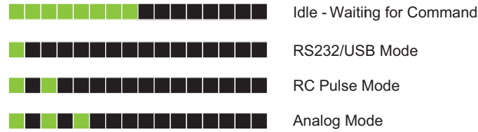
FIGURE 16. Status LED Normal Operation Flashing Patterns
