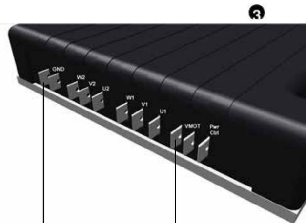
Connect power source V+ to the VMOT connection on drive **3** and the V- to the GND connection on drive **3**
